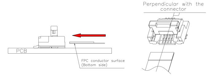
12.1.3 Rotate down the actuator until firmly closed. It is critical that the inserted FFC/FPC is not moved and remains fully inserted.
