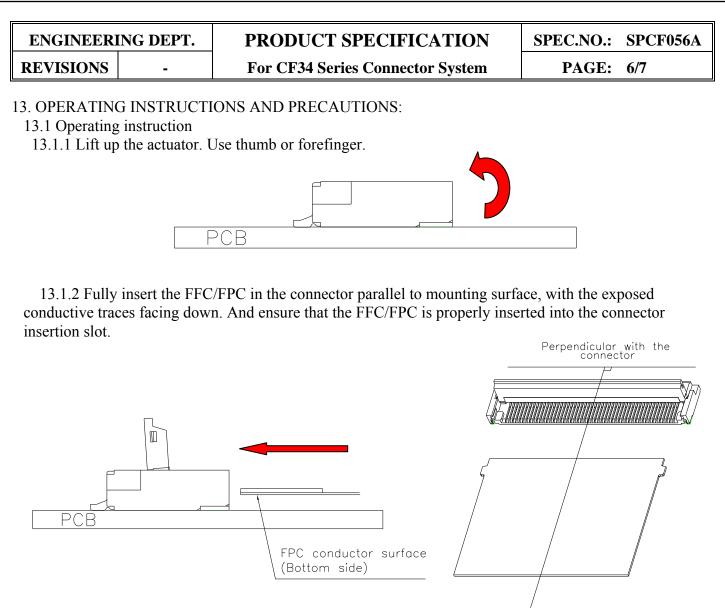
13.1.3 Rotate down the actuator until firmly closed. It is critical that the inserted FFC/FPC is not moved and remains fully inserted.
