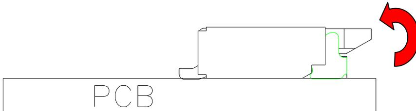
13.1.2 Fully insert the FFC/FPC in the connector parallel to mounting surface, with the exposed conductive traces facing down. And ensure that the FFC/FPC is properly inserted into the connector insertion slot.
