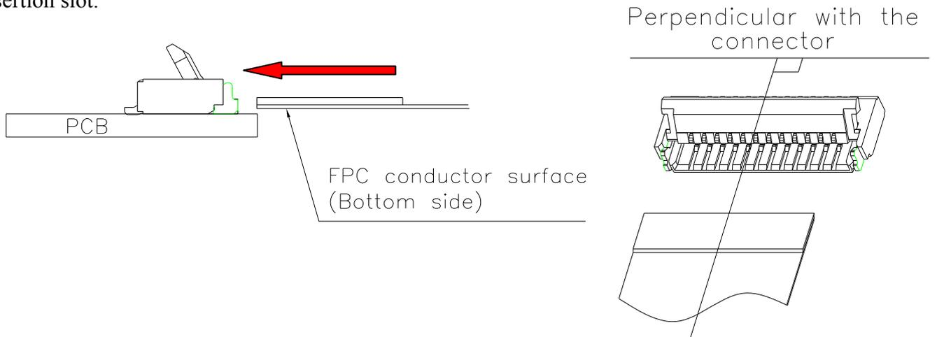
13.1.3 Rotate down the actuator until firmly closed. It is critical that the inserted FFC/FPC is not moved and remains fully inserted.
